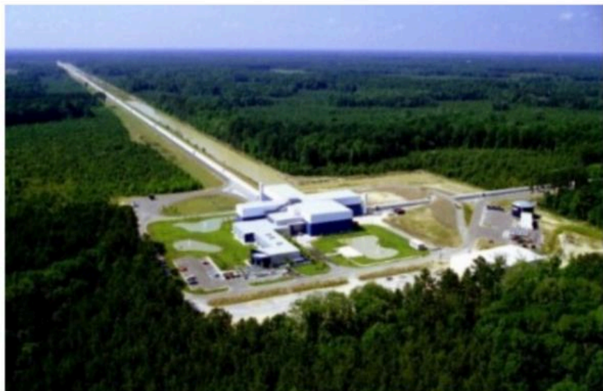
Fig.2.LIGO Livingston-the arms are concrete structures that protect the vacuum tubes which reside just inside
